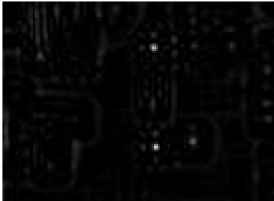
Fig. 6 The correlation surface from the top level of the pyramid is shown. Two strong peaks, representing the location of the two instances of the model, are evident. These peaks provide coarse location estimates, which are refined as the algorithm descends through the pyramid.
