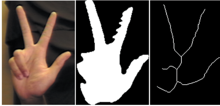
Fig. 12. Successful detection of a 3-finger hand gesture.
