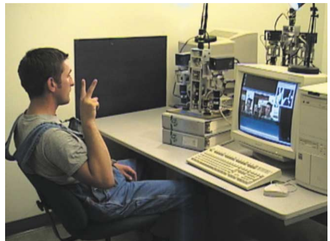
Fig. 2. System setup with two TRISH-2 robotically controlled binocular camera heads. In front of the acting person the receiving system is placed while the affecting system is located in the back (top right corner of the image). The receiving system is monitored on the PC-screen.
