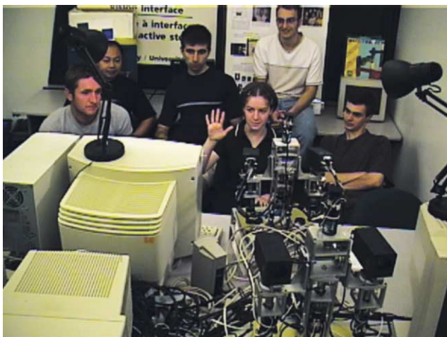
Fig. 14. System setup with two robotically controlled binocular camera heads and an operator who has raised her hand. The system provides robust and reliable results even with cluttered backgrounds.
