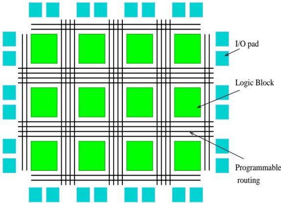
**Figure 1: Architecture of a generic FPGA**
