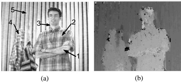
**Figure 10: (a) Input from right camera (b) Output disparity map**
