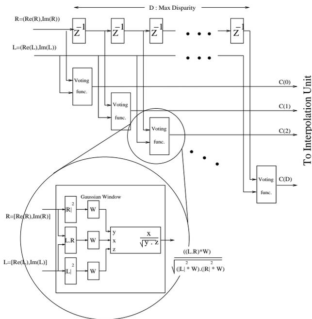
Figure 4: Original correlation block architecture
