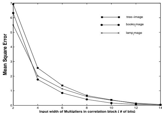
Figure 5(b): Error in final disparity resulted from fixed-point multipliers
