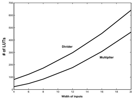
Figure 5(a): Divider and multiplier hardware cost
