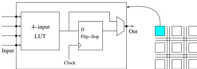
**Figure 2: Simplified architecture of a logic block with one 4-LUT**
