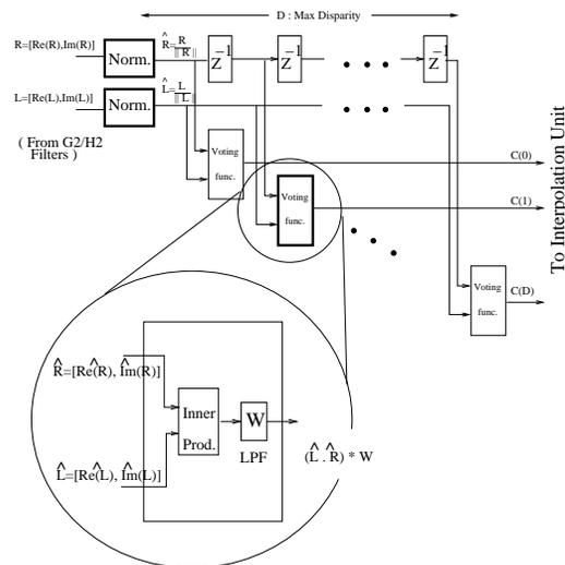
Figure 6: Revised correlation architecture with normalization blocks
