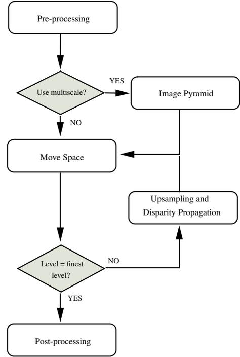
**Figure 2. Flow diagram of multi-resolution graph cuts using stereo-motion constraints system.**
