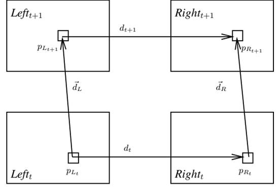
**Figure 1. Example of two stereo image pairs ( $L_t, R_t$ ) and ( $L_{t+1}, R_{t+1}$ ) at times  $t$  and  $t + 1$ , respectively. A point  $p_{L_t}$  in the reference frame  $Left_t$  is related to its corresponding points in the other images via established disparity values  $d_t, d_{t+1}, \vec{d}_L$  and  $\vec{d}_R$  for stereo pairs at time  $t, t + 1$ , left-motion image pairs, and right-motion image pairs, respectively.**
