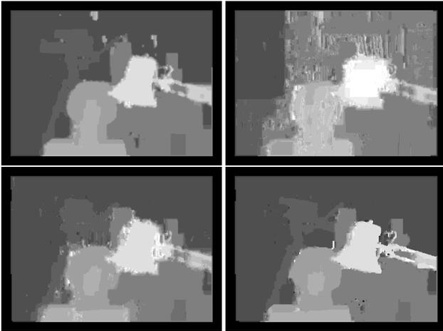
**Figure 8.** The disparity maps for the left motion pair of images: MRGC (top-left), LDNR (top-right), EL (bottom-left), SAC(bottom-right).
