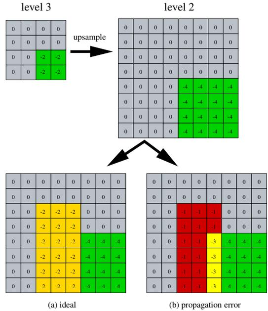
**Figure 4. After upsampling a disparity map from level 3 to level 2, we find the presence of label error propagation between levels of the pyramid. The ideal solution for level 2 should be (a). However, a disparity value of -2 is not in the label disparity neighbourhood of disparity values of 0 or 4. Therefore, using LDNR, the disparity map achieved at level 2 would be as in (b) where the disparity values of -1 (red) and -3 (yellow) are errors that propagate to subsequent levels.**
