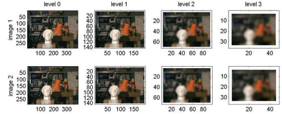
**Figure 5. Image pyramids for an image pair. From left to right, the images proceed up the pyramid, passing from the finest to the coarsest level of the pyramid with each image axis indicating the image dimensions in pixels.**
