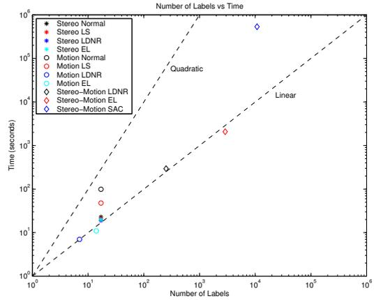
**Figure 7. The relationship between the number of labels used in an algorithm and the time to convergence for all graph cut algorithms (stereo, motion and combined stereo-motion).**
